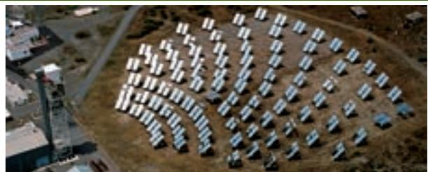
Figura 5. Central experimental de receptor central en la PSA [3].
